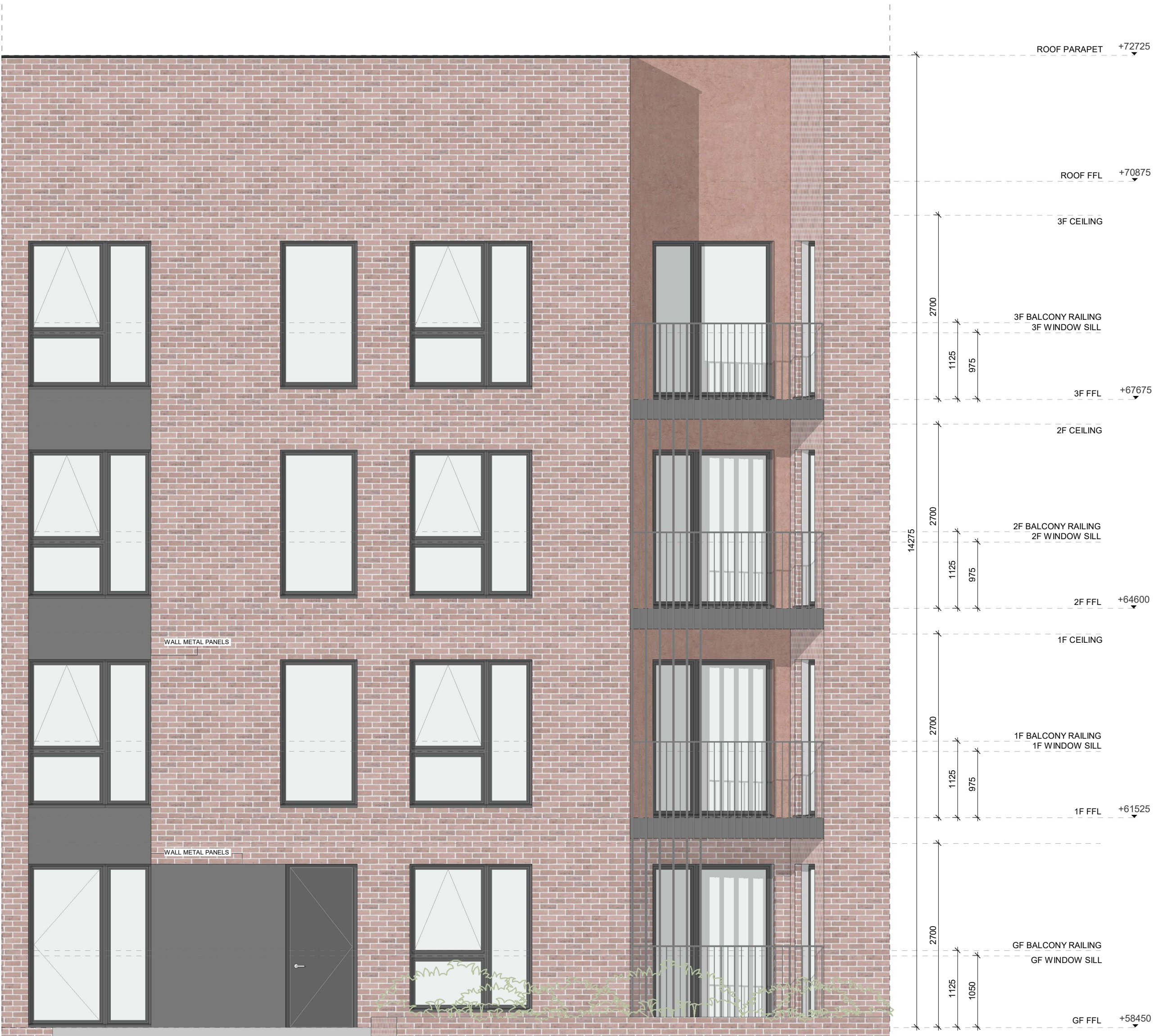
APARTMENT BLOCK H - MATERIALITY - TYPICAL FRONT ELEVATION 1 : 50
